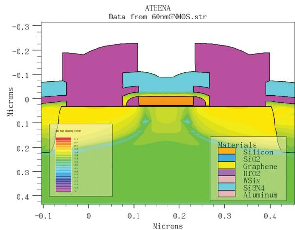
FIGURE 1. Doping profile of graphene field effect transistor
