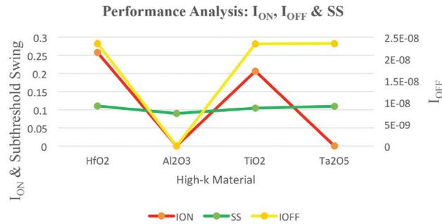
FIGURE 6. Results of  $I_{ON}$ ,  $I_{OFF}$  and SS at different dielectric material
