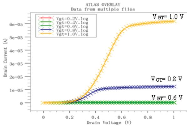
FIGURE 5.  $I_D$ - $V_D$  of GFET at different  $V_{GT}$
